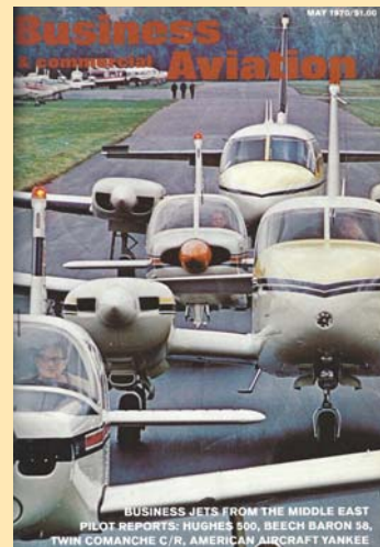
Indian-file on the taxiway at Lock Haven, Pennsylvania, for of Piper's best-selling models pose for photographer Simpson Kalisher. The line-up, foreshortened in the long lens, shows a Cherokee followed by an Aztec D, Cherokee Arrow and a Navajo. Of the aircraft shown, only the twins are built in Lock Haven; all Cherokees are built at the company's Vero Beach, Florida, plant.
