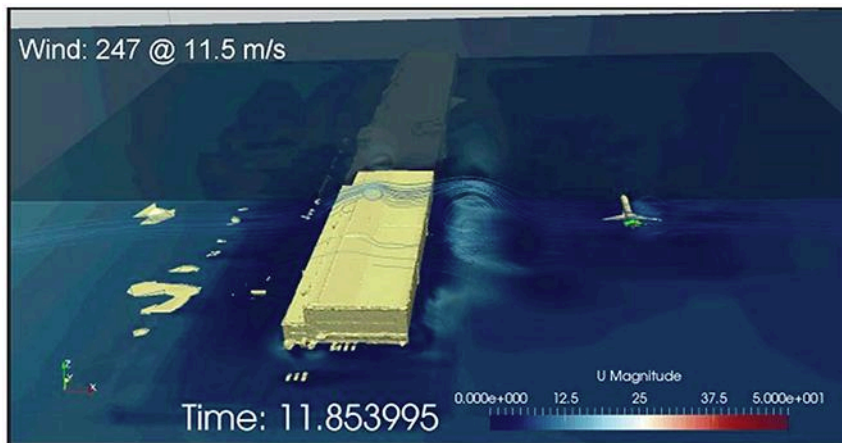
3-D visualization of wind simulation results for a discrete time showing the locations of the hangar and airplane. Wind flow from the west (left side) is disrupted downwind of the hangar.
