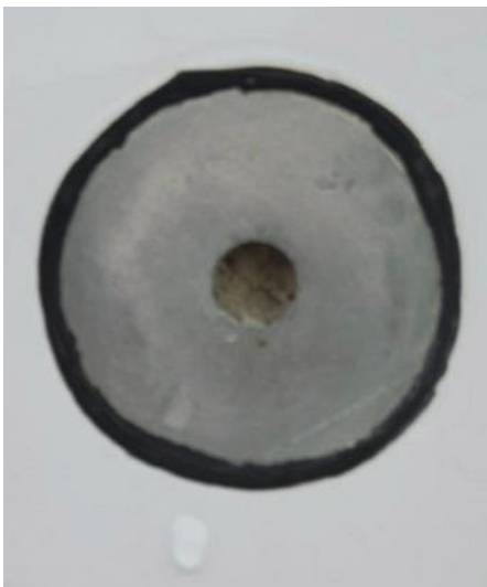
Close-up of the outflow valve static port.
