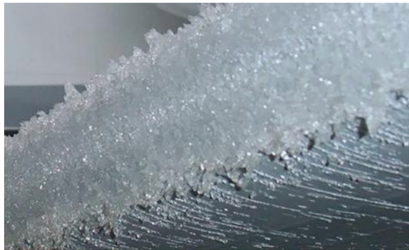
The ice accretion was about 4 cm wide and had a milky, rough, crystalline appearance and a slightly concave form.
