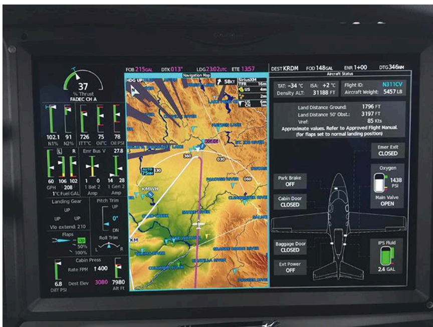
Photographic proof of performance claims. FL 310, 309 KTAS at ISA+5C on 37% thrust. EFIS screens are the sharpest in the aviation industry, symbol colors are unambiguous, synthetic vision is standard.
