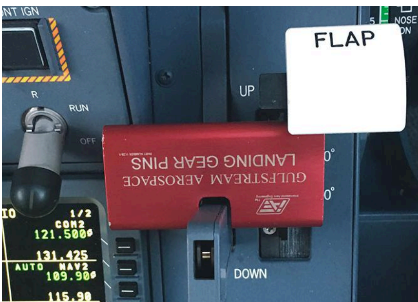
Gulfstream gear pin holder installed between the gustlock and flap handles.
