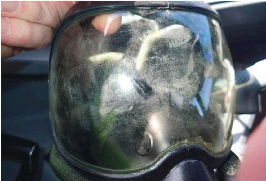
Copilot's smoke goggles showing obscuring layer on inner surface.
