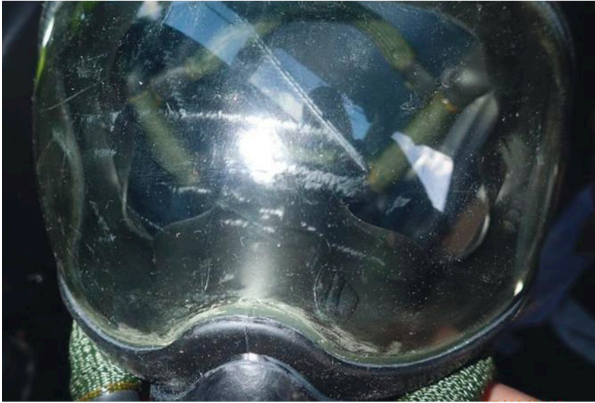
Exterior of pilot's smoke goggles showing scratches.
