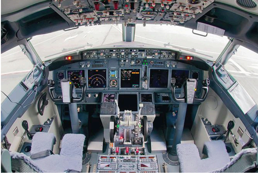
Cockpit features six LCD screens, standard Collins HUD, triple IRS, CAT III-capable flight guidance system, FANS-1/A equipment, ADS-B-out and full-feature FMS. WAAS LPV and ADS-B-IN are not offered.
