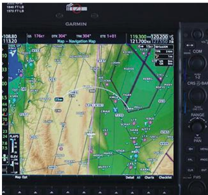
Displays may be configured as full screen, as show above, or split screen with a moving map and an electronic chart of checklist.
