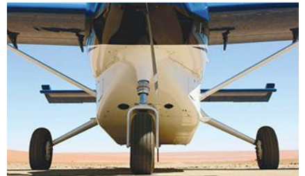
Beefier optional heavy-duty landing gear affords a 565-lb. boost in operating weights.
