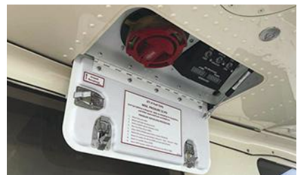
Optional single-point pressure refueling virtually is a must when aircraft is fitted with floats.
