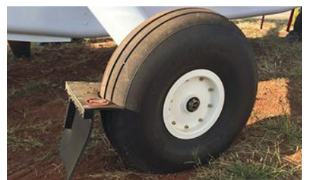
Optional mud flaps help prevent ravel and stone damage to horizontal stabilizer.
