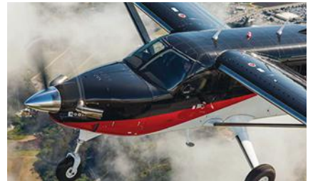
Sixteen-gallon TKS system protects prop, windshield and wings. It's replaced by a hydraulic power pack when the aircraft is fitted with floats.
